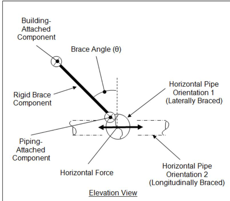
3.2.2 Figure 3.2.2A Typical Brace Layout, Horizontal Pipe
