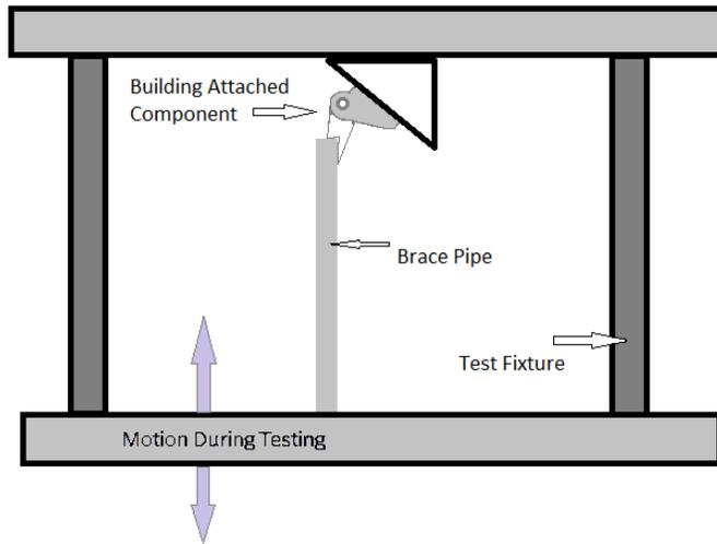
4.2.1 Figure 4.2 – Building Attached Subassembly, 30° Orientation
