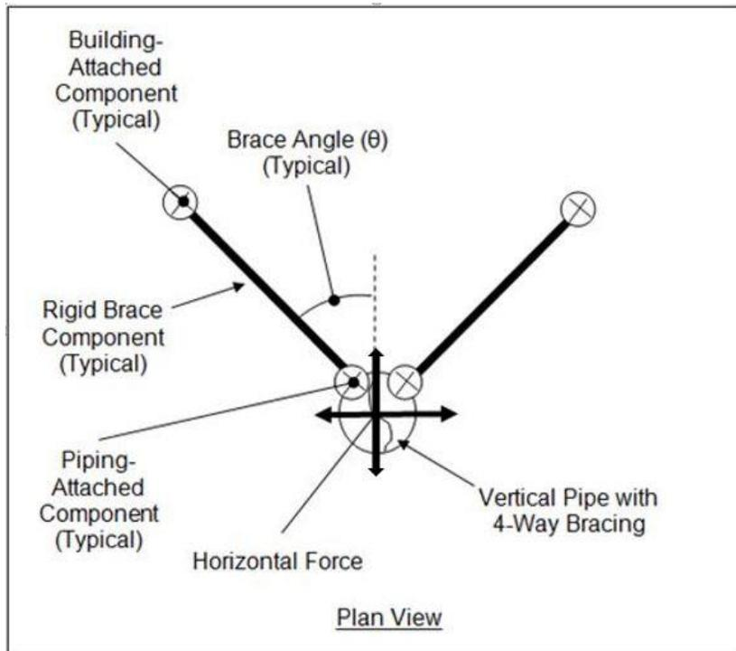
3.2.3 Figure 3.2.2B Typical Brace Layout, Vertical Pipe
