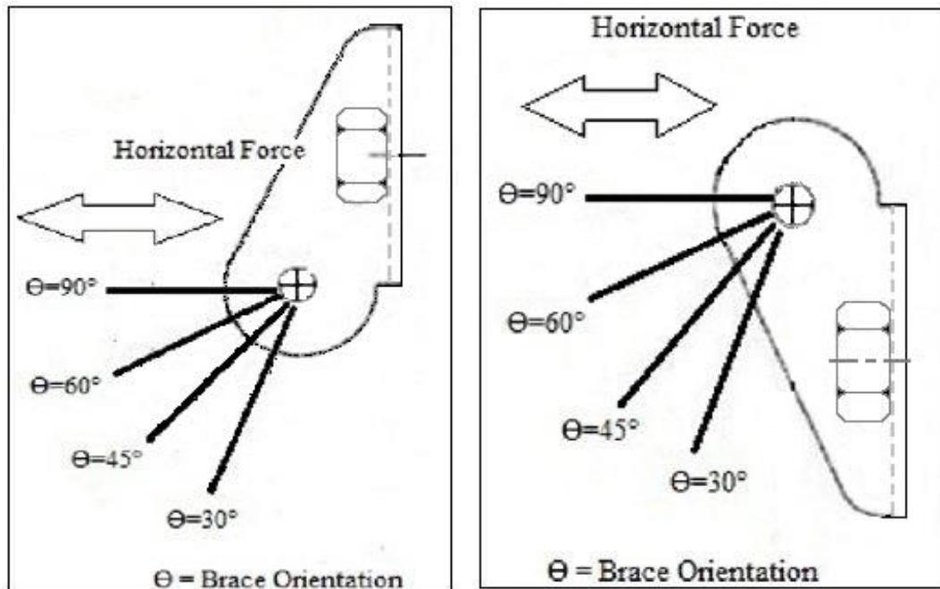
4.2.3 Figure 4.2.3B – Building-Attached Component with Side Attachment to Wall or Beam
