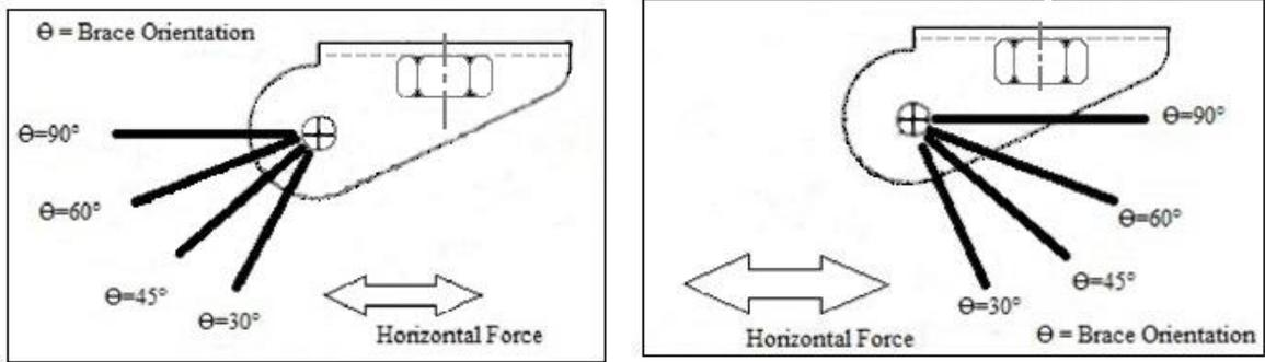
4.2.2 Figure 4.2.3A – Building-Attached Component with Overhead Attachment to Floor or Beam
