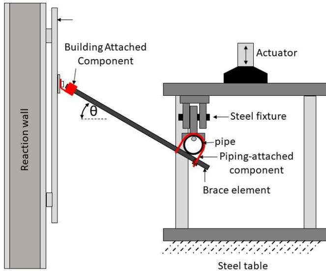
Figure 4.3.2 Test Arrangement for Assembly Testing
